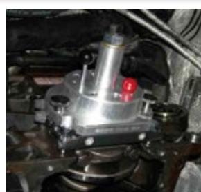
**VW CRAFTER 2.5 TDI Common Rail****Device for the exchange of the shaft seal****Art. 911 325 00**
